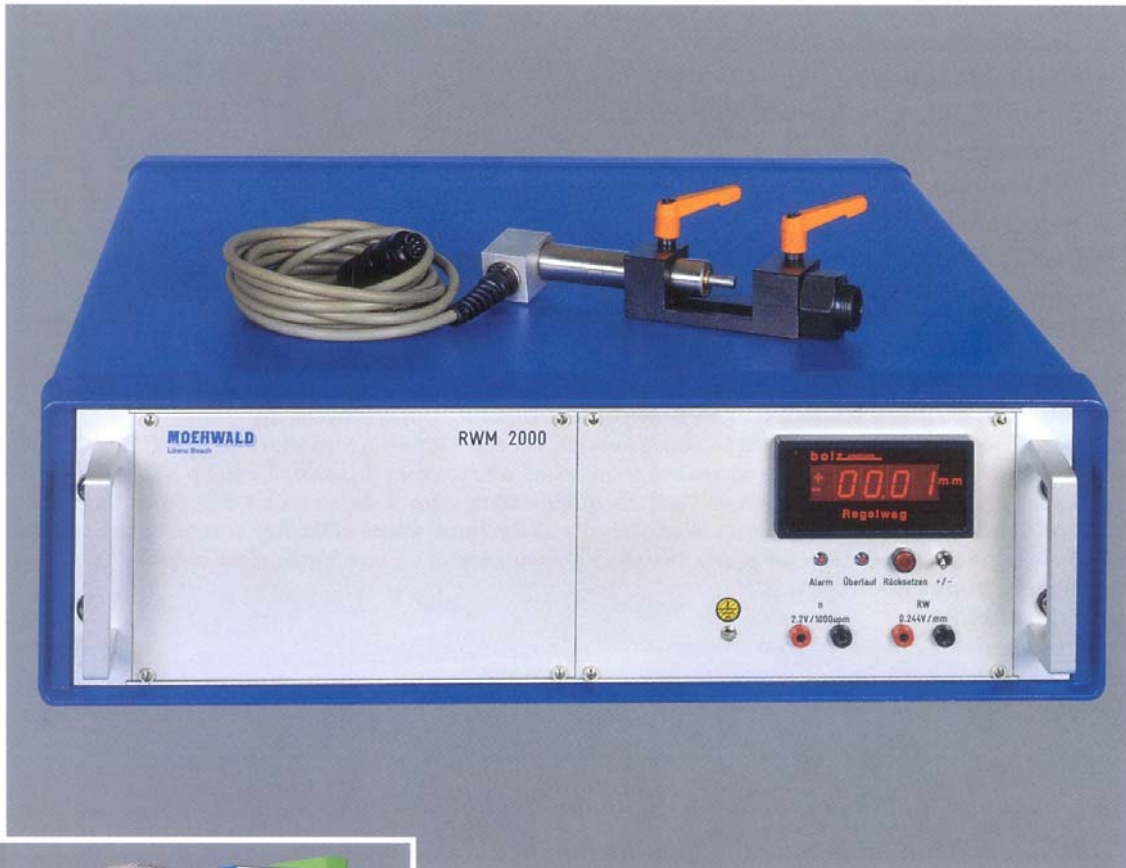
Control rack travel measuring device with magnetic encoder and optional control rack travel holder
