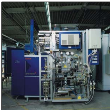
Hydraulics and instrumentation completely onboard
