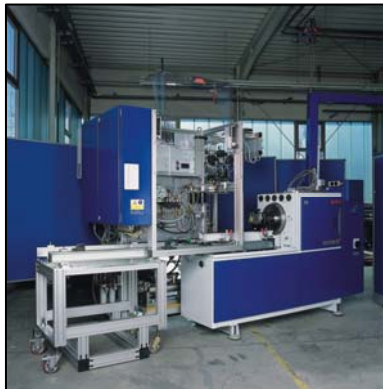
Easy mounting by means of wheeled carrier and quick adapters
