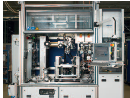
Flexible single production and development test bench CGI 4000 for common rail injectors
