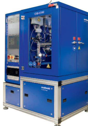
Test bench CRI 4000 for common-rail injectors R&D and series testing (medium and heavy duty)
